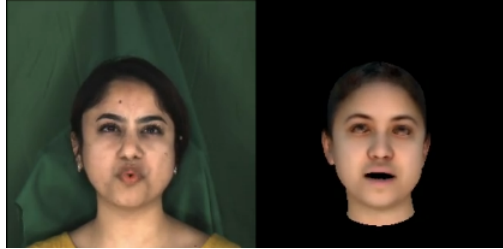
Figure 2: An example of a typical failure in the monocular reconstruction method. ( Left ): The input frame, ( right ): the reconstruction. Note how FLAME model lacks the expressiveness to capture certain mouth shapes, in this case an "O".
